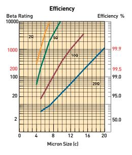
Notes: Multipass test run @ 80 l/pm to 3.5 bar terminal - 5 mg/l BUGL.
