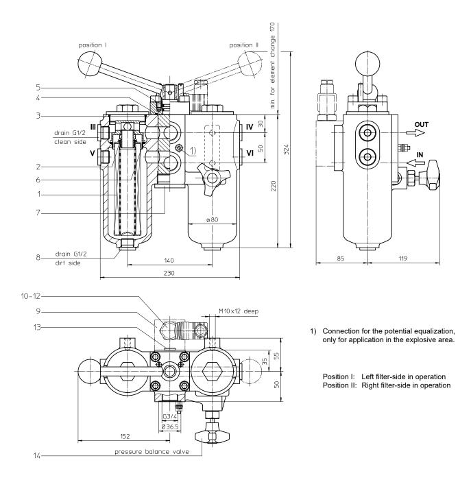
Measuring connection III, IV: Drain G  $^{1\!\!/}_2$  - clean side Measuring connection V, VI : Air bleeding, pressure relief G  $^{1\!\!/}_2$  - dirt side
