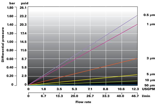
\* For liquids other than water, multiply pressure drop by fluid viscosity in centipoise.
