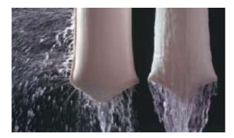
These photos clearly demonstrate the dramatic advantage of the weld liquid filter bag over coventional sewn seam bags. Conventional sewn seams contain needle holes that measure up to 1200 micron.
