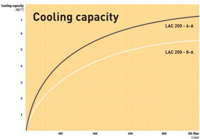
Cooling capacity tolerance  $\pm$  10% kW.
